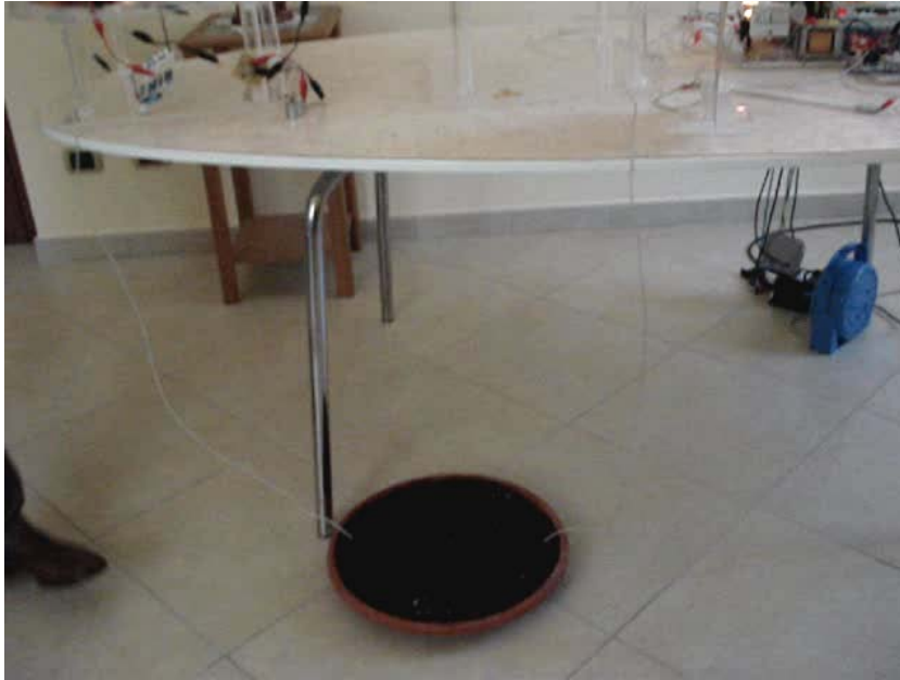
Figure 3: connection through the ground of the two flat spiral Tesla Coils
