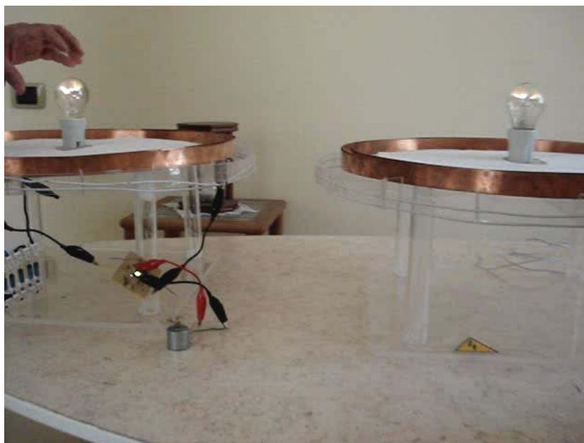
Fig. 2: Tesla coil (XMTR and RCVR) connected through the ground.
